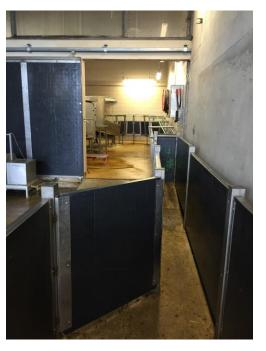
Welded Construction - Steel Quality S235 - Hot Galvanized Finish according to EN ISO 1461 2009
