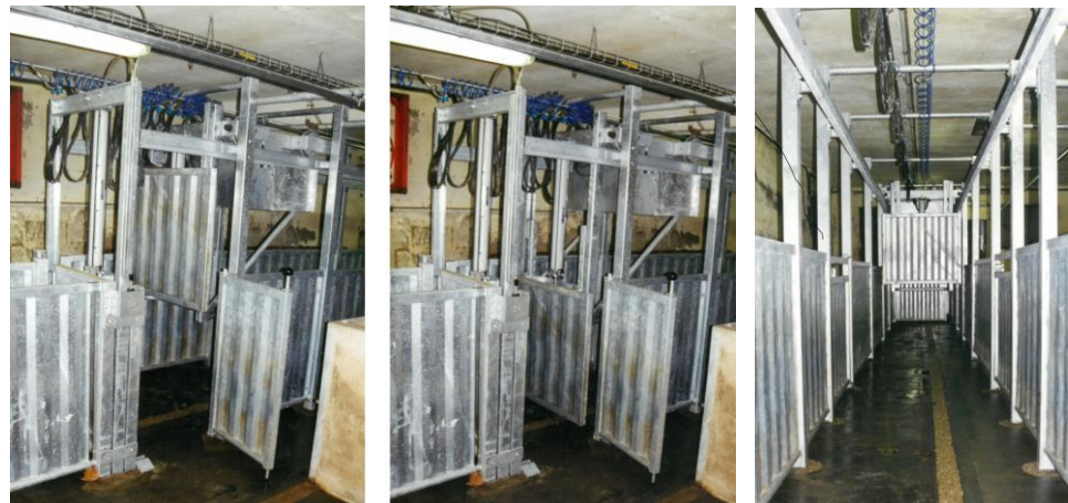
The electric rolling door and pneumatic sash allow adjustment of the available space as the animals move onto the anaesthesia line.
