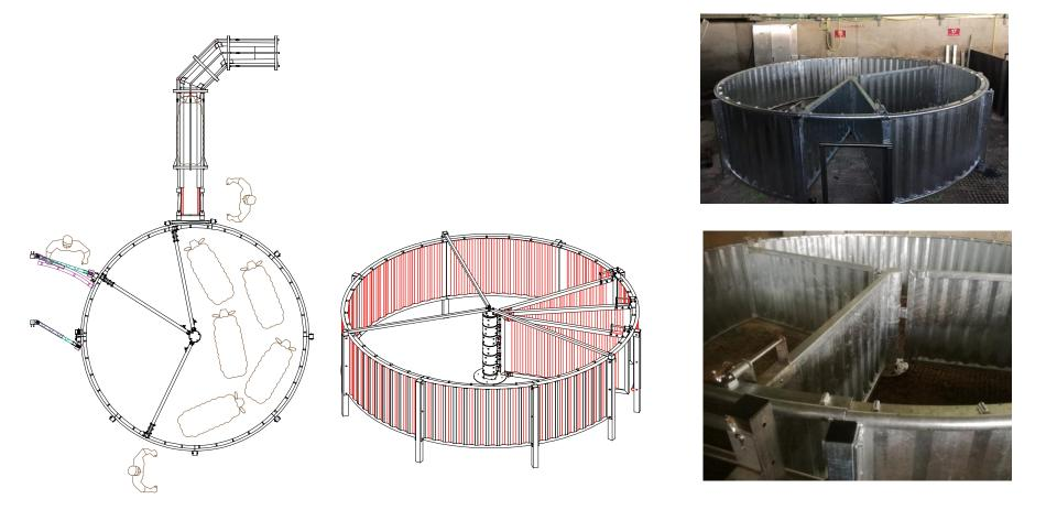
Welded Construction - Steel Quality S235 - Hot Galvanized Finish according to EN ISO 1461 2009
