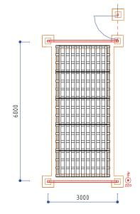
Depth ± 750 Peripheral rebate 240 x 125 Rainwater connection
