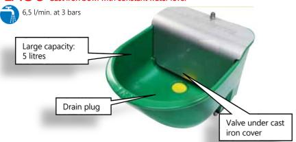
Connection to horizontal  $\frac{34}{7}$  (20x27) tube below. Connection to vertical  $\frac{1}{2}$  (15 x 21 mm) tube below possible (using accessory brass fitting 55 mm)
