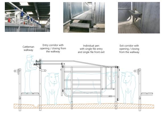
Noncontractual Welded Construction - Steel Quality S235 - Hot Galvanized Finish according to EN ISO 1461 2009
